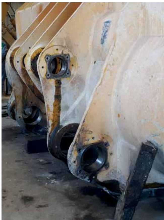
Komatsu 600 series Front End Loader in for maintenance where Thordon's ThorPlas-Blue bearings will be installed
