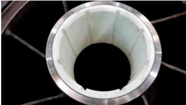
Thordon's SXL bearings installed in KSB three-stage mixed flow impeller-type pumps
