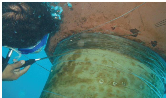
Aft shaft seal damage caused by fishing net caught in the propeller
