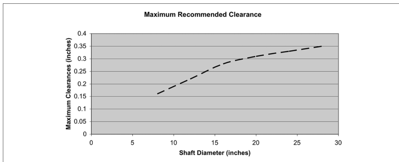
Figure 21: Typical Maximum Clearance (imperial) for Stern Tube and Strut Bearings
