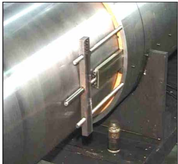
Figure 4. Single Key removal using key extraction tool
