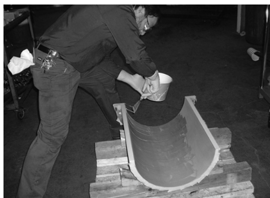
Figure 5: Adhesive applied to split metal housing.
