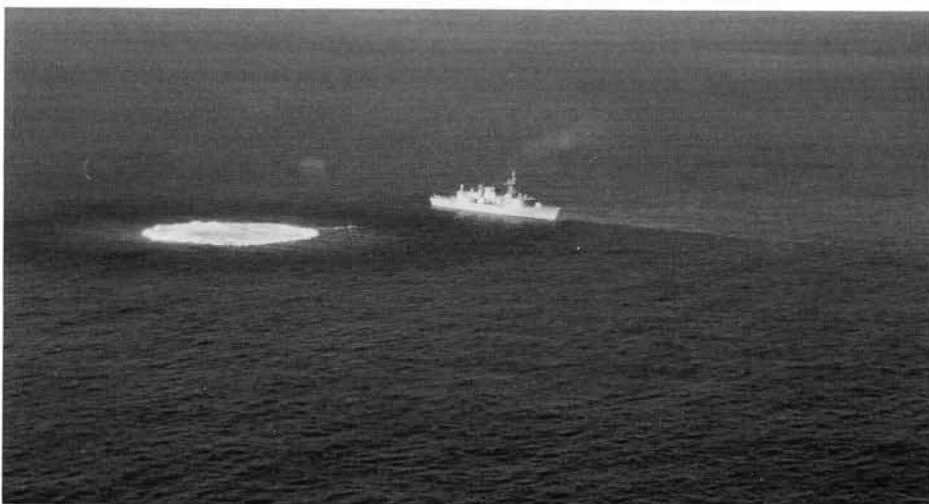
Shot 3: The big one. This series of photos taken from one of the helicopters shows the effects of the initial shock wave reaching the surface ( top ), the formation of the plume ( centre ), and the formation of a three-metre surface wave. ( CFB Halifax photos )
