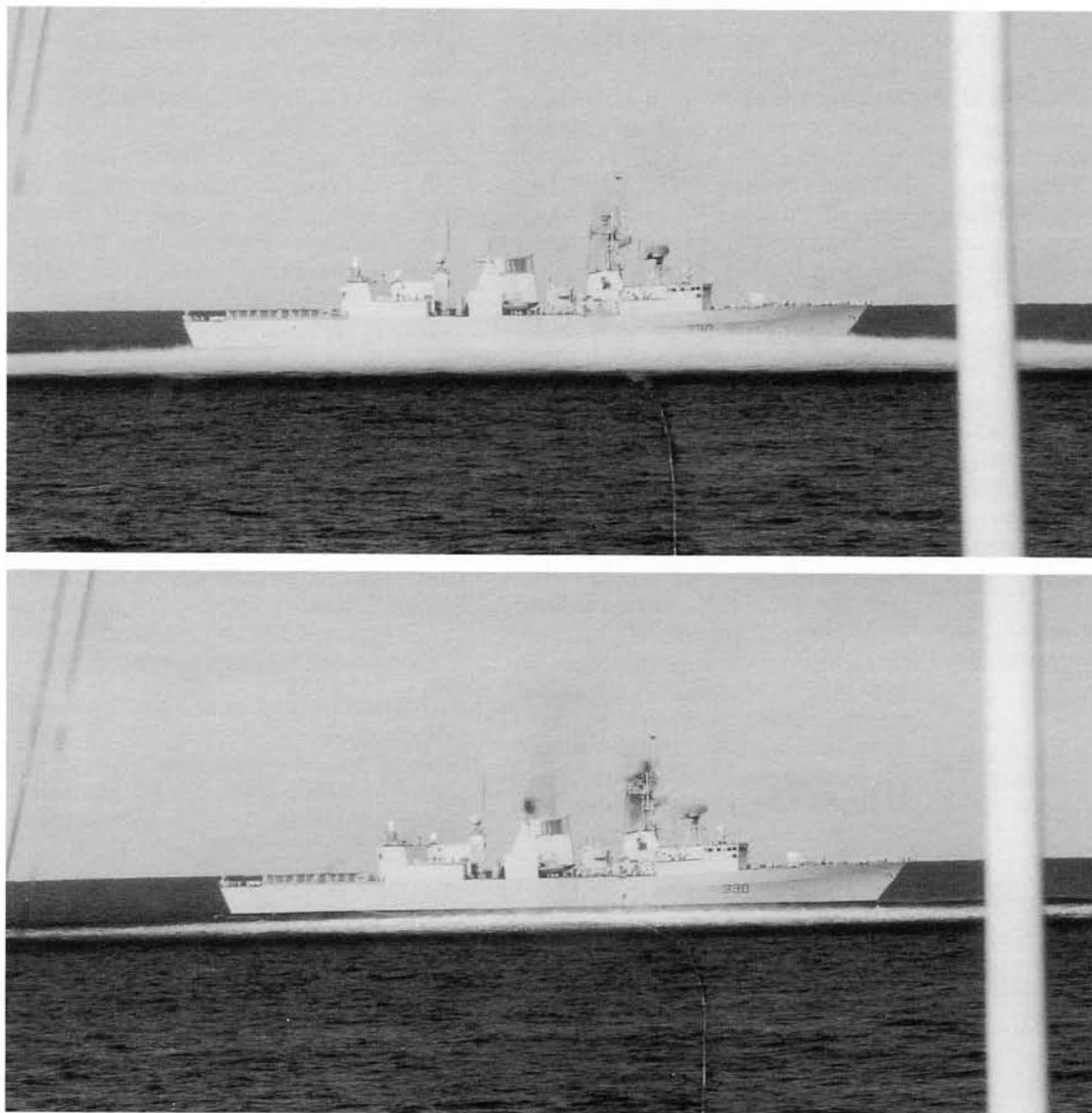
Fig. 6. Shot 3: As viewed from Riverton , five tonnes of high-explosive were used for the final test in the CPF shock qualification program. The charge geometries were designed to apply uniform keel and hull shock factors along the length of the entire ship. (CFB Halifax Base Photo)
