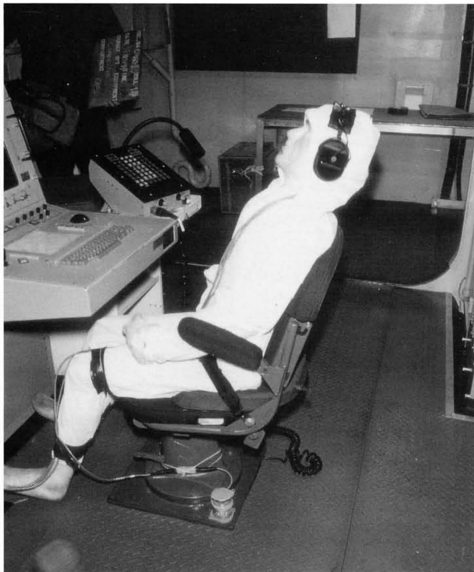
Veterans of numerous personnel vulnerability investigations, mannequins such as this one in Halifax's operations room were fitted with triaxial accelerometers to measure shock response. The gauge on the deck below the seat monitored the shock input. (NETE photo by George Csukly)
