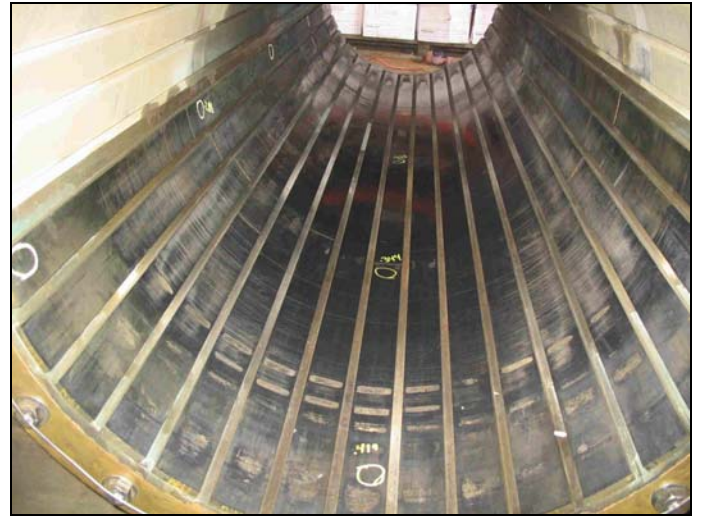
Photo 6 - Aft Sterntube Bearing – Looking Aft
