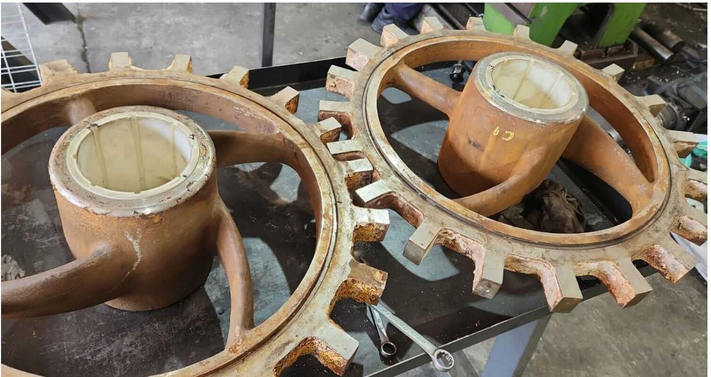
Thordon SXL installed in the spider housings for Sulzer fire pumps.
